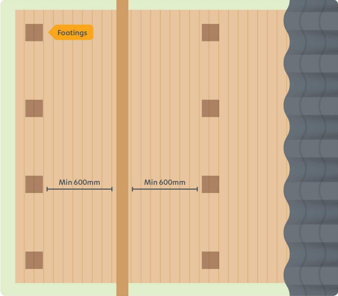
Figure 11: Garage over gravity sewer supporting a habitable structure
