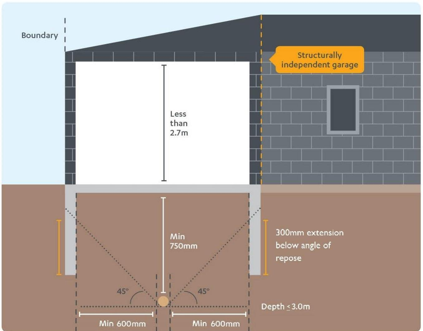
Figure 13: Garage adjacent gravity sewer
