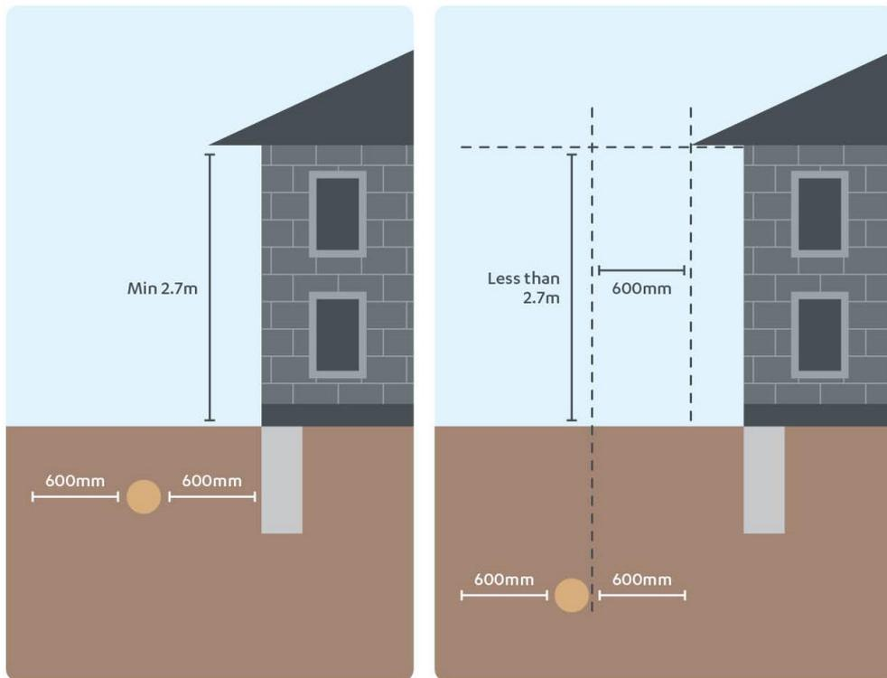
Figure 22: Balconies and over-hangings over sewers greater than 3 m deep
