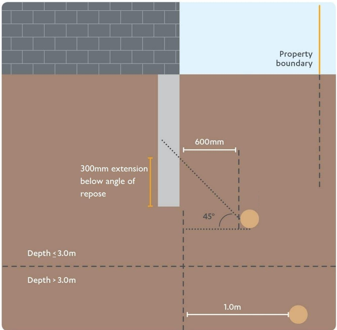
Figure 3: Cantilevered habitable structure
