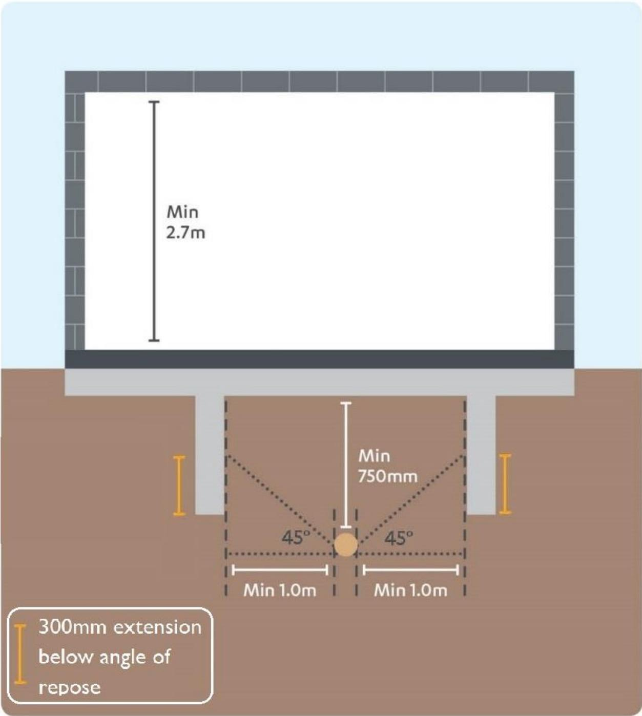
Figure 8: Footing requirements for commercial property adjacent gravity sewer
