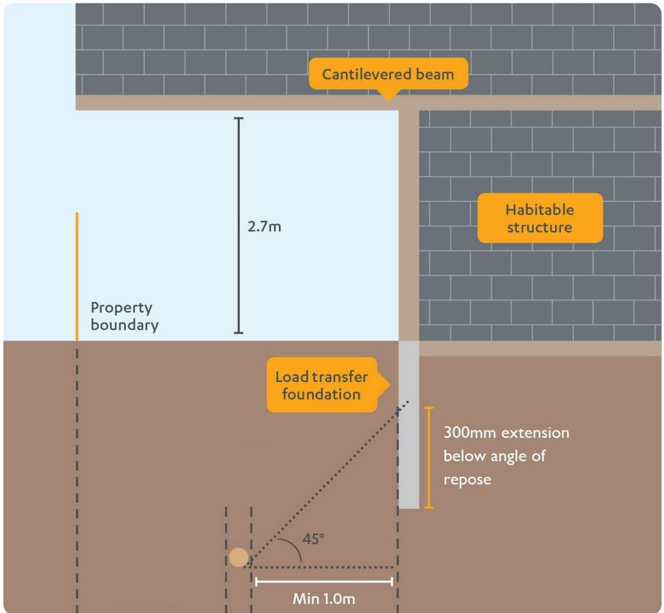
Figure 4: Control zone of manholes, maintenance shafts and end of lines
