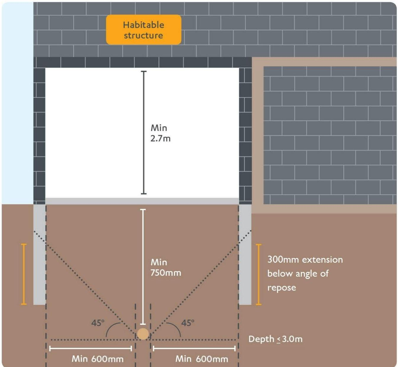
Figure 12: Garage with height clearance less than 2.7 m and over gravity sewer
