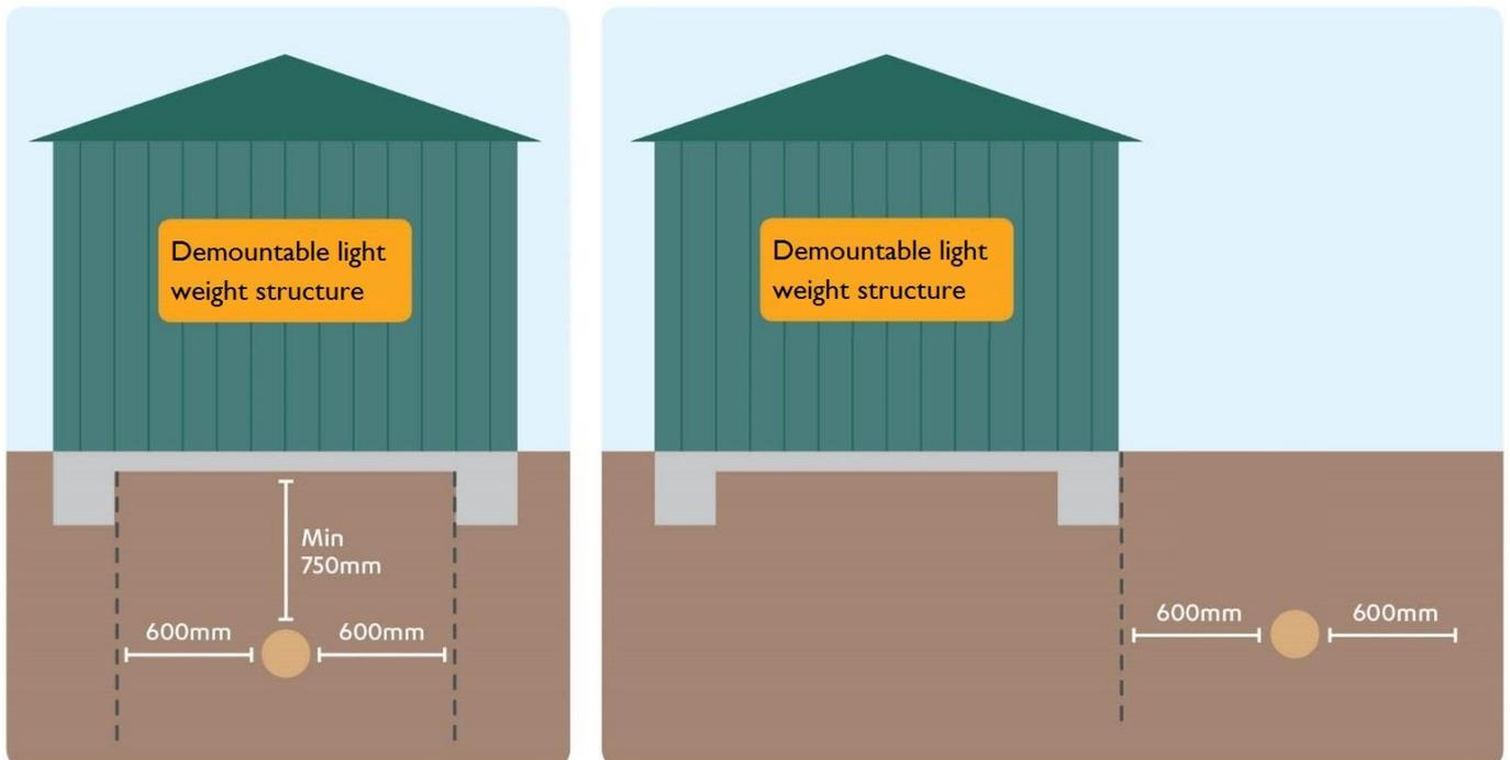
Figure 10: Decking over sewer
